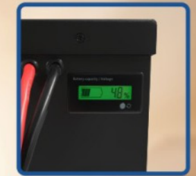
Battery Status Display
