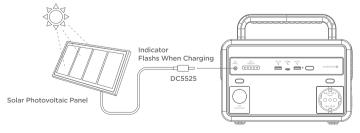
Note: The solar charging voltage is 12V-26V, the open circuit voltage needs to be lower than 26V, and the maximum input power is 100W.
